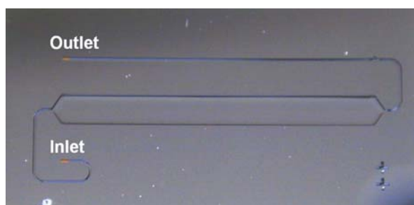
Figure 2. Microfabricated reactor after anodic bonding with colloids inside. The gas inlet and outlet are seen in the left side of the picture.
